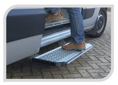
The **VERSA SL** is made from a combination of steel and aluminium, and weighs between 16Kg to 18 Kg the **VERSA SL** is mounted below the middle sliding door. With a deployment time of 1.5 seconds, the **VERSA SL** step will keep up with fast paced activities and regular use. The tested life cycle of the step is 250,000 cycles. This ensures the durability and reliability we know you need. A high temperature zinc corrosion protector is also used to increase the durability.
