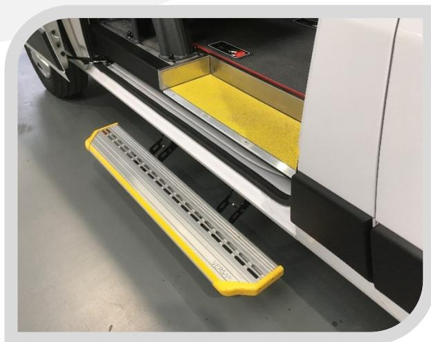
The **VERSA SLC 1000** is made from a combination of steel and aluminium, and weighs 12 Kg the **VERSA SLC 1000** is mounted below the middle sliding door. With a deployment time of only 1.5 seconds, the **VERSA SLC 1000** step will keep up with fast paced activities and regular use. The tested life cycle of the step is 250,000 cycles. This ensures the durability and reliability we know you need.
